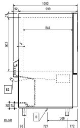
Drain Electrical inlet (power) FΙ Refrigerant Outlet
